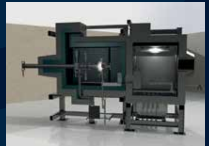
Beamline End Cell for high Energy Pelletron line, Dalton Institute
